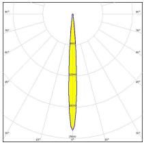
Dimensions: 74.7 mm x mm Height: 42.80 mm ~15° spot beam
