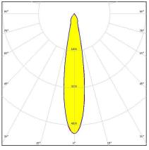
Dimensions: 74.7 mm x mm Height: 42.80 mm ~24° medium beam
