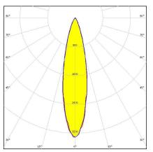
Dimensions: 34.0 mm x 34.0 mm Height: 10.70 mm ~25° medium beam
