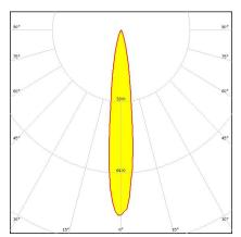
Dimensions: 34.0 mm x 34.0 mm Height: 10.70 mm ~12° spot beam
