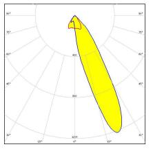
Dimensions: 279.5 mm x 39.6 mm Height: 20.30 mm Asymmetric beam for aisle lighting. Clear version for high contrast lighting.
