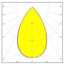
**Dimensions: mm x mm Height: mm** ~50° wide beam with tighter cutoff. Variant with diffused lenses.
