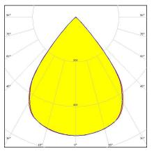
Dimensions: 279.5 mm x 39.6 mm Height: 20.30 mm ~80° wide beam. Variant with diffused lenses.
