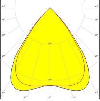
Dimensions: 19.0 mm x 259.0 mm Height: 40.00 mm ~80° batwing beam
