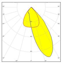
Dimensions: 279.5 mm x 39.6 mm Height: 20.30 mm Asymmetric beam for aisle lighting.
