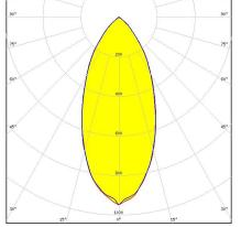
Dimensions: 279.5 mm x 39.6 mm Height: 20.30 mm ~35° wide beam. Variant with diffused lenses.
