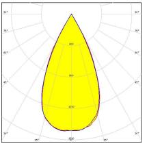
Dimensions: 279.5 mm x 39.6 mm Height: 20.30 mm ~50° wide beam with tighter cutoff
