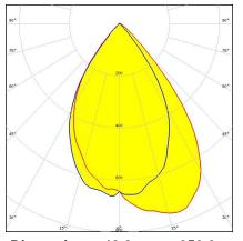
Dimensions: 40.0 mm x 259.0 mm Height: 20.30 mm Forward throwing beam for freestanding office luminaires
