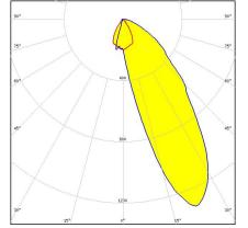
Dimensions: 279.4 mm x 40.0 mm Height: 27.00 mm Asymmetric beam for wall-washing
