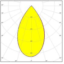
Dimensions: 279.5 mm x 39.6 mm Height: 20.30 mm ~50° wide beam. Variant with diffused lenses.
