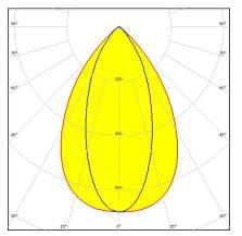
Dimensions: 279.5 mm x 39.6 mm Height: 20.30 mm ~25 + 70° oval beam. Variant with diffused lenses.
