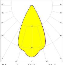
Dimensions: 90.0 mm x 90.0 mm Height: 16.89 mm ~50° wide beam. New revision.
